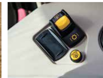
Operator control comes from the switch mounted on the right-hand console
